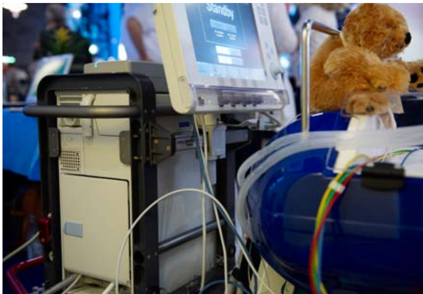
The ventilator is securely mounted to the stretcher by means of a special transport cage, which maintains stability throughout the flight.
