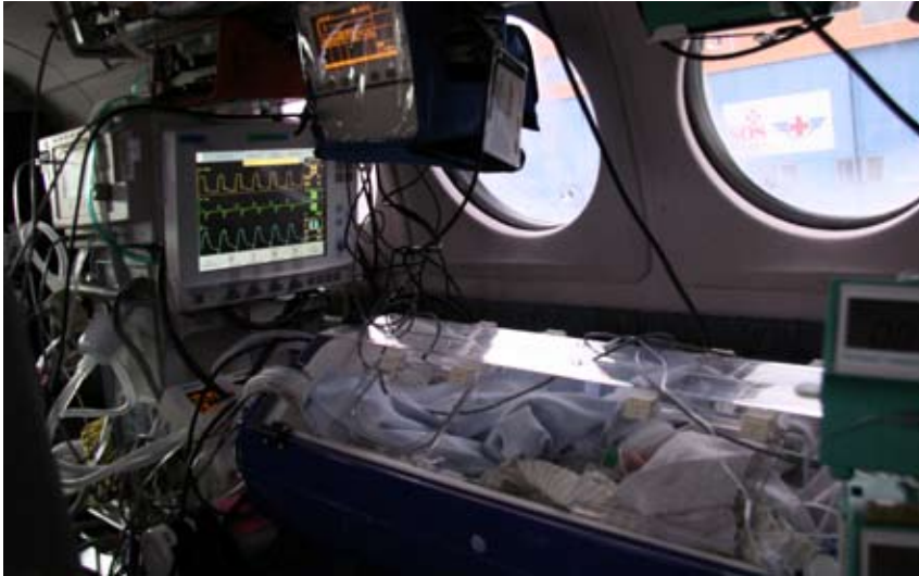
The single unit concept, with ventilator and infant pod attached to the same stretcher, has increased ease-of-use and minimized risks, according to staff members.
