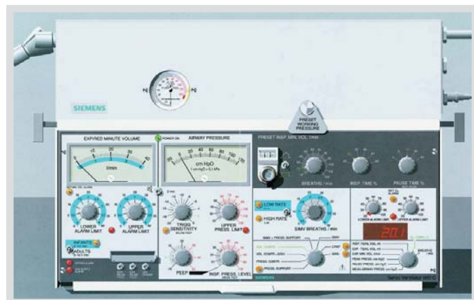
The SERVO 900C was the first mechanical ventilator to offer the Pressure Support mode.
